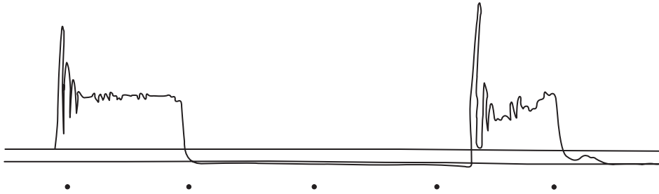
Fig. 1. Pressure record exhibiting column separation. Horizontal axis: time (each dot indicates half a second). Vertical axis: pressure (Joukowsky pressure of 15.3 bar). The upper horizontal line is the static pressure and the lower horizontal line is the atmospheric pressure. [Adapted from Joukowsky (1900, Fig. 17); also shown by Simin (1904, Fig. 13), and by Moshnin and Timofeeva (1965, Fig. 1)].
